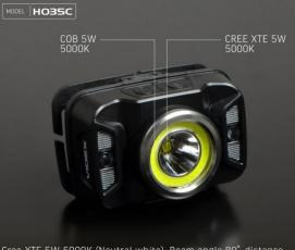
Cree XTE 5W 5000K (Neutral white). Beam angle 80°, distance up to 86 m. COB 5W 5000K (Neutral white). Beam angle 120°, distance up to 14 m.
